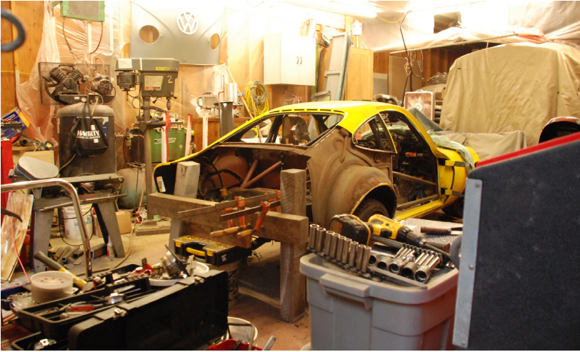
Using various clamps and timber we were able to straighten the rear beam.
