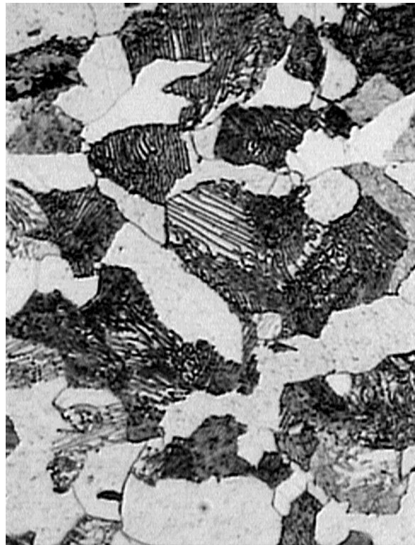
Figure 2. The necklace structure in 1045 steel. As this material cooled from the austenite region the ferrite (light) formed first at prior austenite grain boundaries and pearlite (lamellar) formed later in the remaining material.
