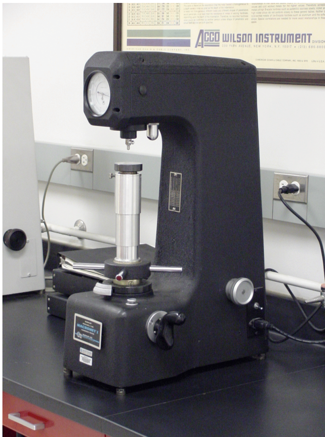
Figure 1 The Buehler Macromet I manual Rockwell-type hardness tester in the materials science laboratories.
