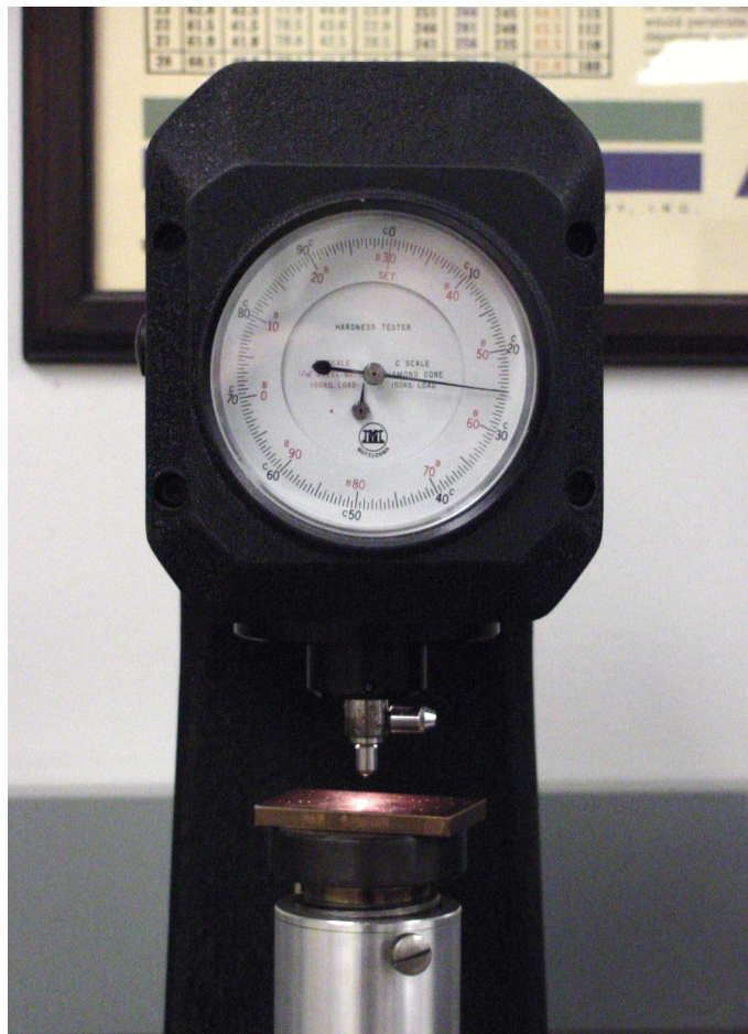
Figure 3 Close-up of the Macromet I's readout dial, indenter and a specimen, in this case a Rockwell B-scale test block.
