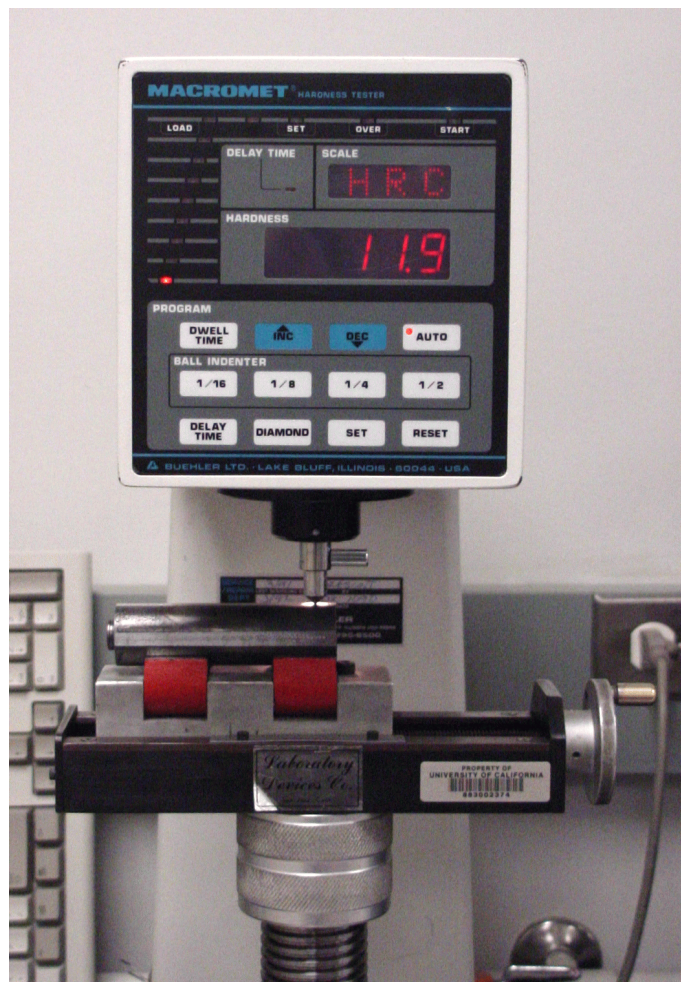
Figure 3 Hardness testing a Jominy specimen. A special Jominy fixture is being used to hold the specimen.
