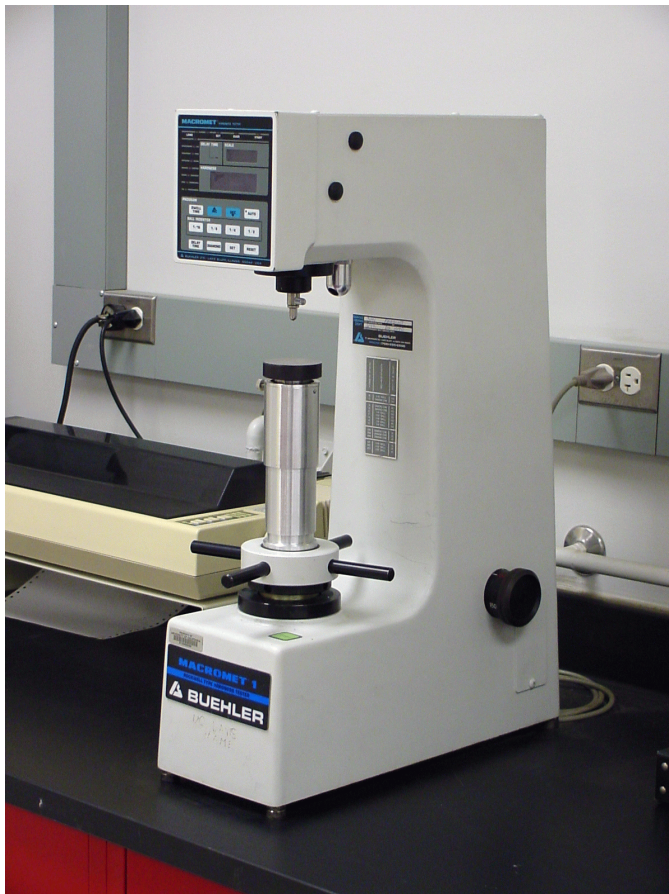
Figure 1 The Buehler Macromet 1 semi-automatic Rockwell-type hardness tester in the materials science teaching laboratories.
