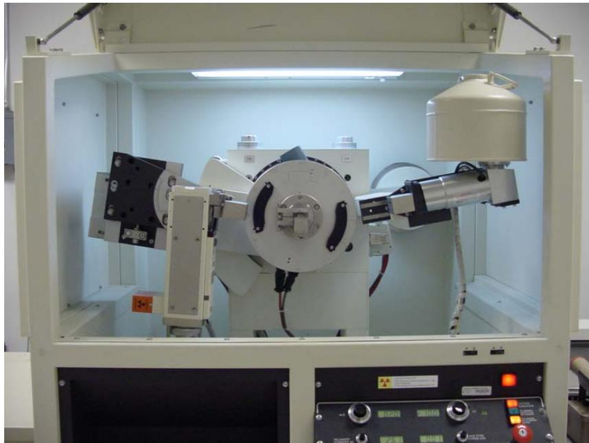
**Figure 1** The Scintag x-ray diffractometer.
