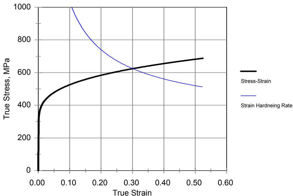
Figure 3. Stress-strain and rate of strain hardening curves calculated using the Hollomon equation (K=500 MPa, n=0.3)
