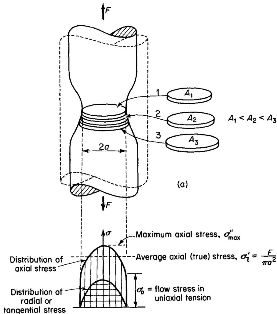
Figure 4. Distribution of stresses in the necked region of a tensile specimen [3].
