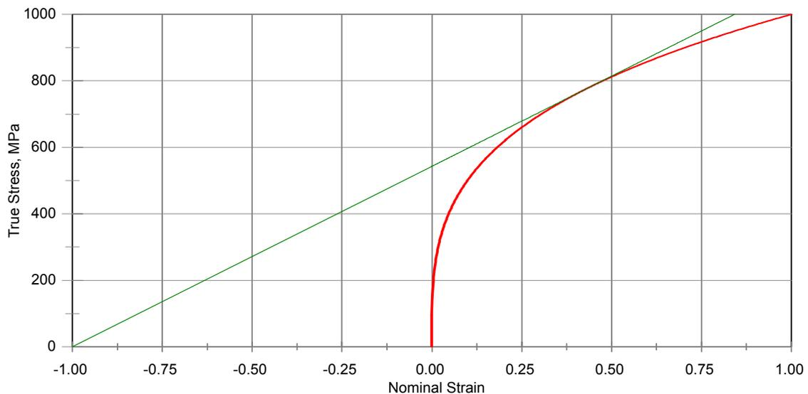
Figure 2. Considère's construction for determining the tensile strength of a ductile material. The tensile strength is found at the intersection of the straight line and the stress axis at strain=0. [2]
