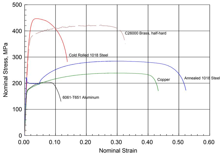
Figure 1. Stress-strain curves for several common alloys.
