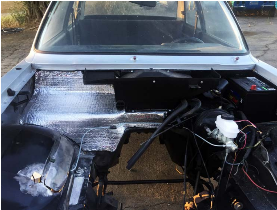
Before putting the engine back in I needed to repair the big hole in the inner fender.
