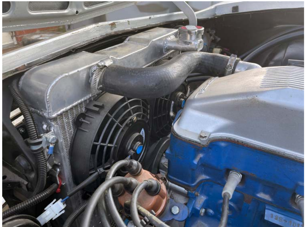
The solution to the radiator fan problem was to install two small fans.
