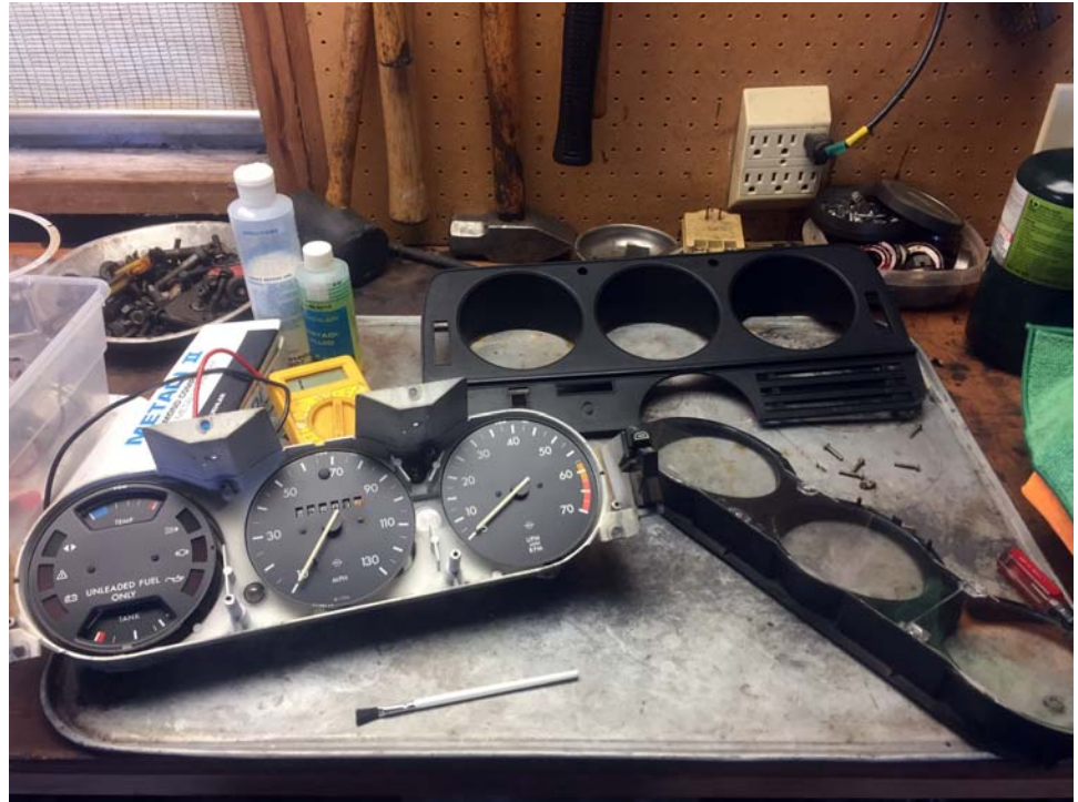
The instrument cluster got a good cleaning and inspection, and LED lights. After replacing the left-most gauge, everything bench tested good.
