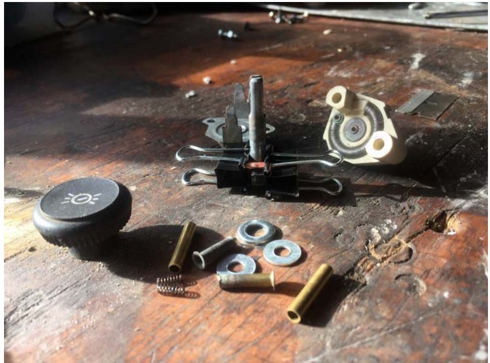
It took some doing, but I got the dimmer apart, made the repairs, then found some brass tubing that fit and managed to get it all back together, and working. Not all car repairs involve a wrench.
